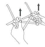
Push the Pivot Grips upwards to raise the height. Squeezing of the Height Adjustment Levers is not necessary.
