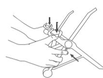
Upon first opening the stand, the height is set at the highest setting. Squeeze the Height Adjustment Levers and push down on the Pivot Grips simultaneously to adjust it to the desired height.
